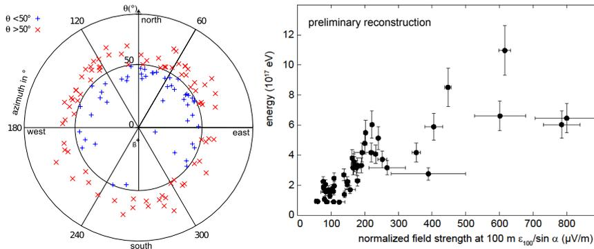
Fig. 2. **right:** Correlation of the reconstructed amplitude of the electric field at 100 m distance to the shower core with the reconstructed energy of Tunka-133. **left:** Event distribution of the preliminary analysis of Tunka-Rex on the sky and the magnetic field direction. Note the asymmetry between north and south sky, as expected from a geomagnetic emission mechanism.
